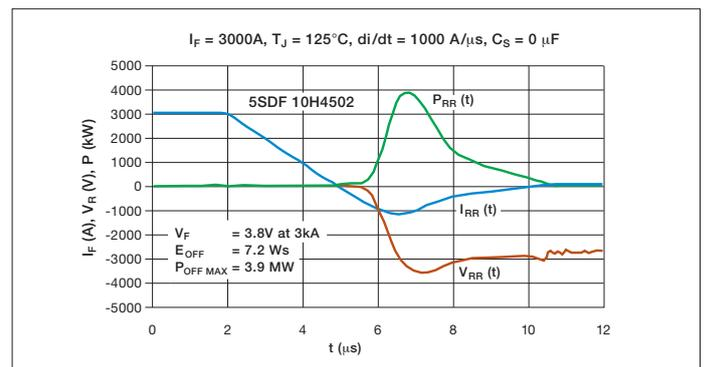
Fig. 1 Snubberless, clamped, FWD commutation showing high SOA and soft recovery
