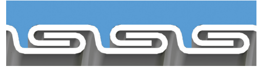
Interlocked Design 1-1/2" through 3" with no bonding wire
