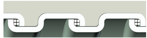
Square-Locked Design with cord packing 3/8" through 1-1/4"
