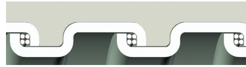
Square-Locked Design with cord packing 5/16" through 1-1/4"
