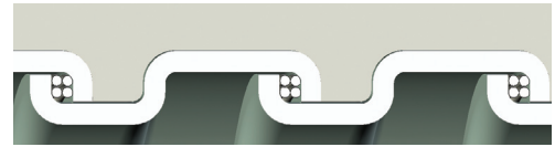
Square-Locked Design with cord packing 3/8" through 1-1/4"
