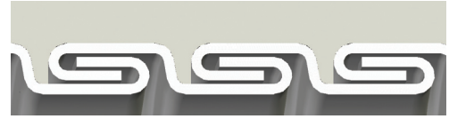
Interlocked Design 1-1/2" through 4" with no bonding wire
