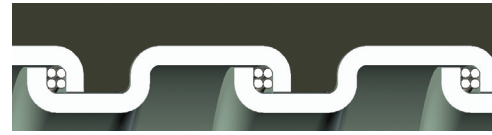
Square-Locked Design with cord packing 3/8" through 1-1/4"
